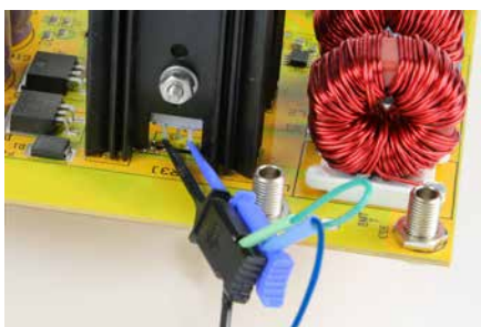
Proper connection using micro-grippers.
