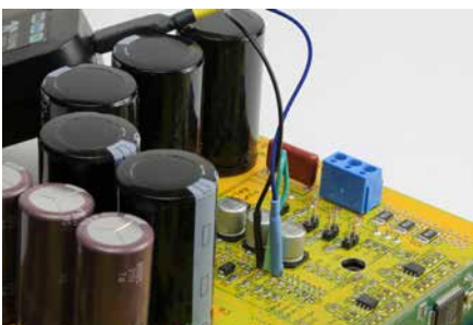
Proper connection using stubs.
