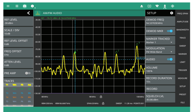
AM and FM Demodulators Play Continuously During Spectrum Sweeps
