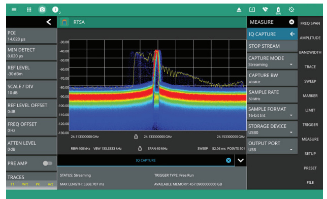
Continuous Update of the RTSA is Supported even When Streaming IQ Data
