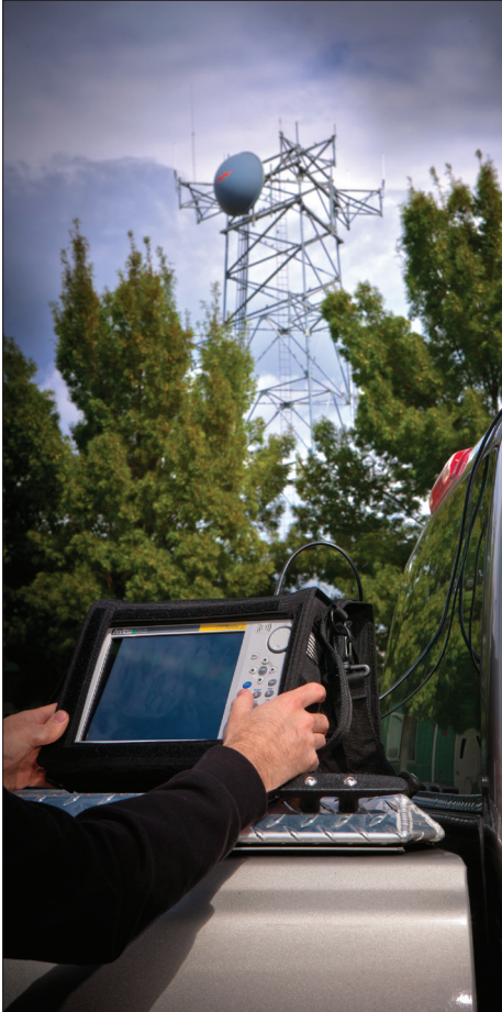
LMR Master Testing from a Service Vehicle
