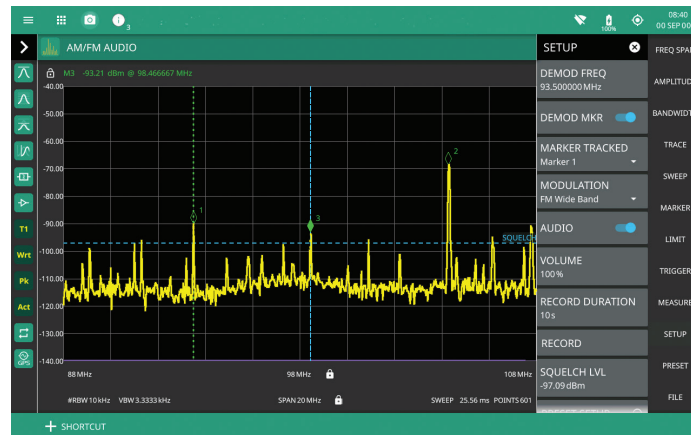
AM/FM Signal Demodulation at Marker Frequency
