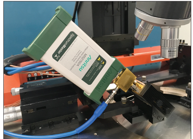
Figure 5. The Spectrum Master MS276xA is Connected Close to the Probe Tip on a Wafer Probe Station
