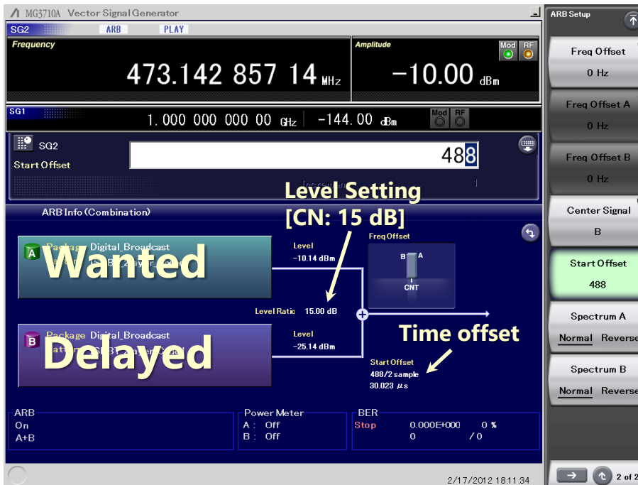
MG3710E Settings for Wanted Signal + Delayed Signal
