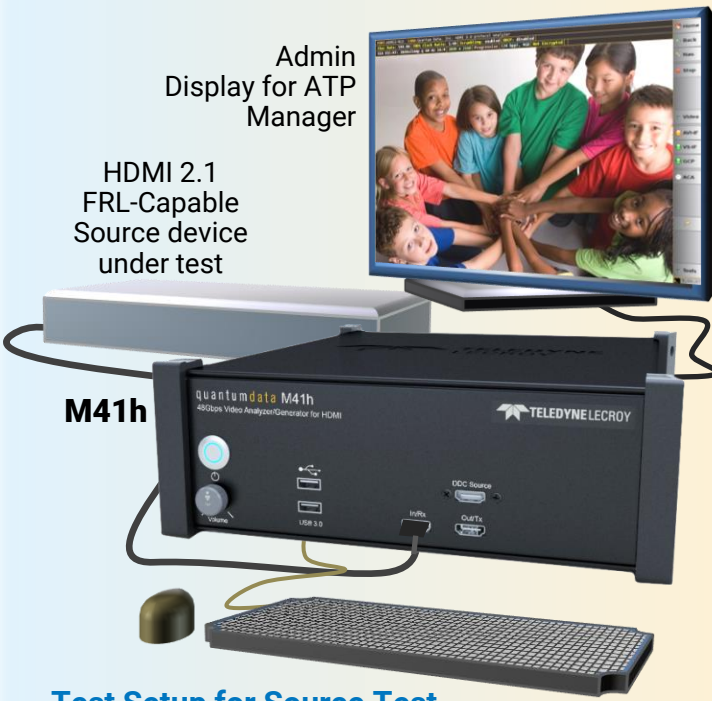
Test Setup for Source Test
