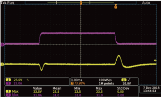
Standalone unit IT6006B-500-30 500V 30A 6000W Setting: voltage 100V current 28A Load current: 30A
